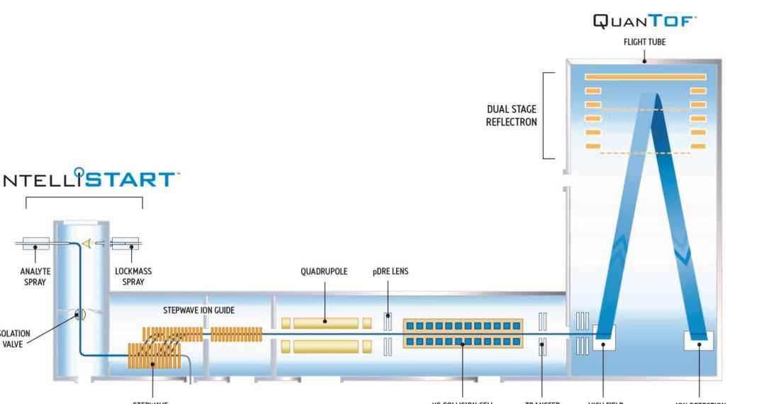
Figure 2. Schematic of the Xevo G2-XS mass spectrometer used for SONAR™ data acquisition
