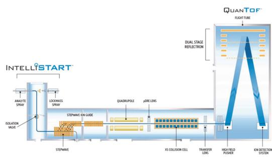
Figure 2. Schematic of the Xevo G2-XS mass spectrometer used for SONAR™ data acquisition
