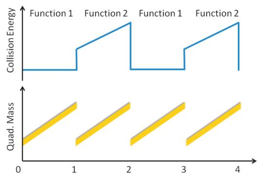
Figure 3. SONAR™ acquisition method and DIA acquisition parameters used in the different experiments.
