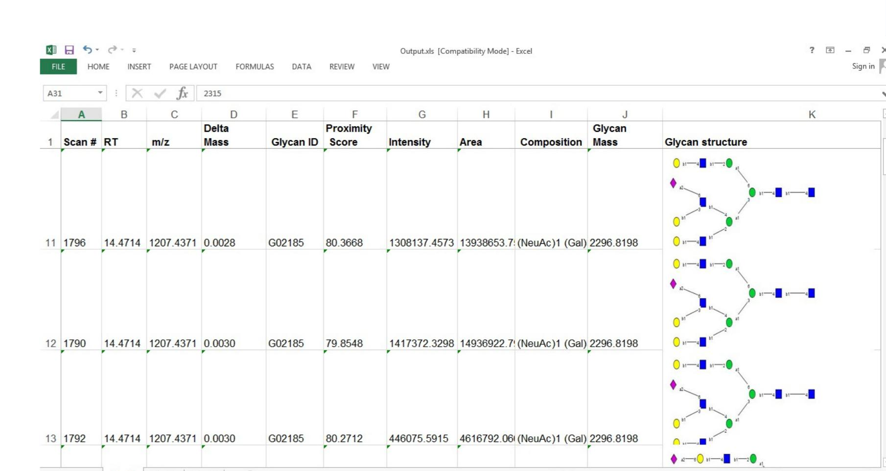
Figure 10: SimGlycan software search result pane; results sorted based on retention time. Identified glycan structures, corresponding fragment ions can be viewed besides corresponding database information.
