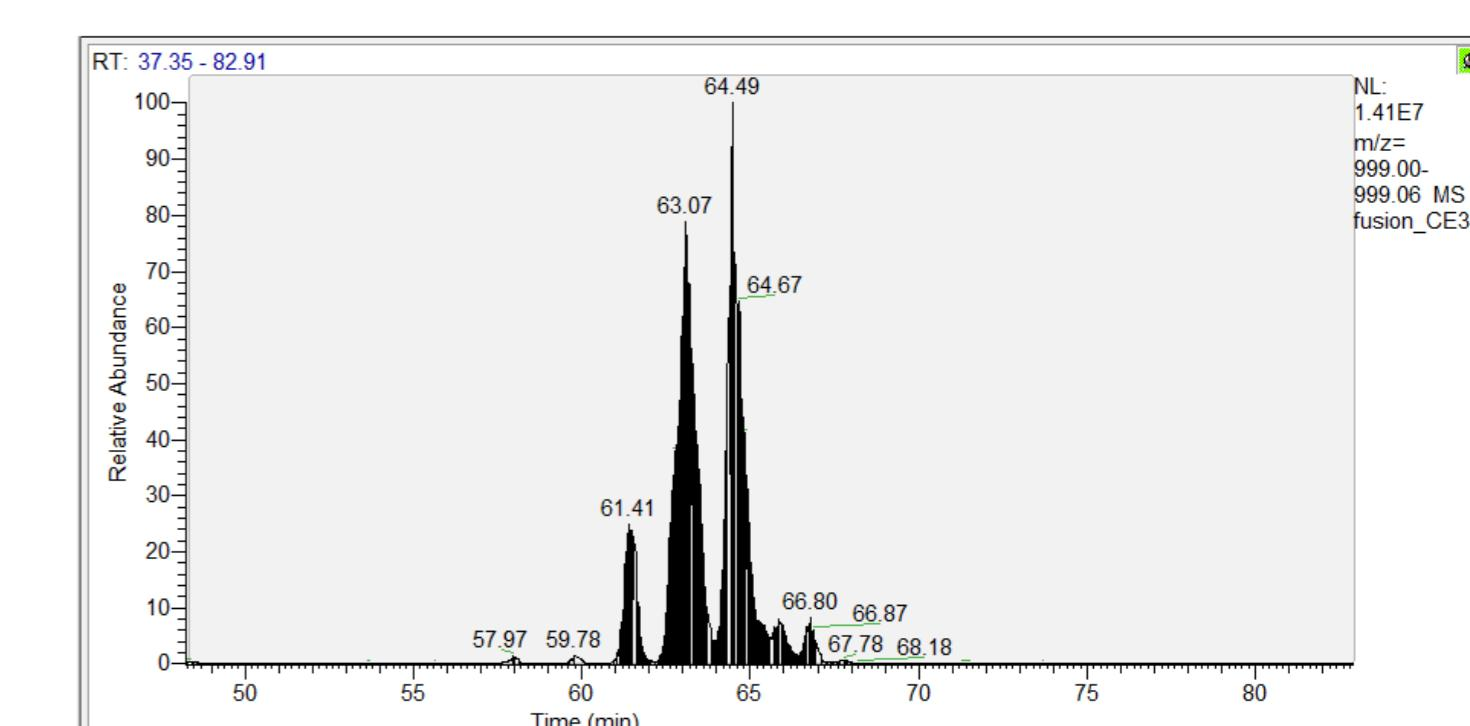
Figure 2: Xcalibur software showing extracted ion chromatogram of 2-AB labelled N-Glycan with precursor  $m/z$  value 998.68 (charge: 3).
