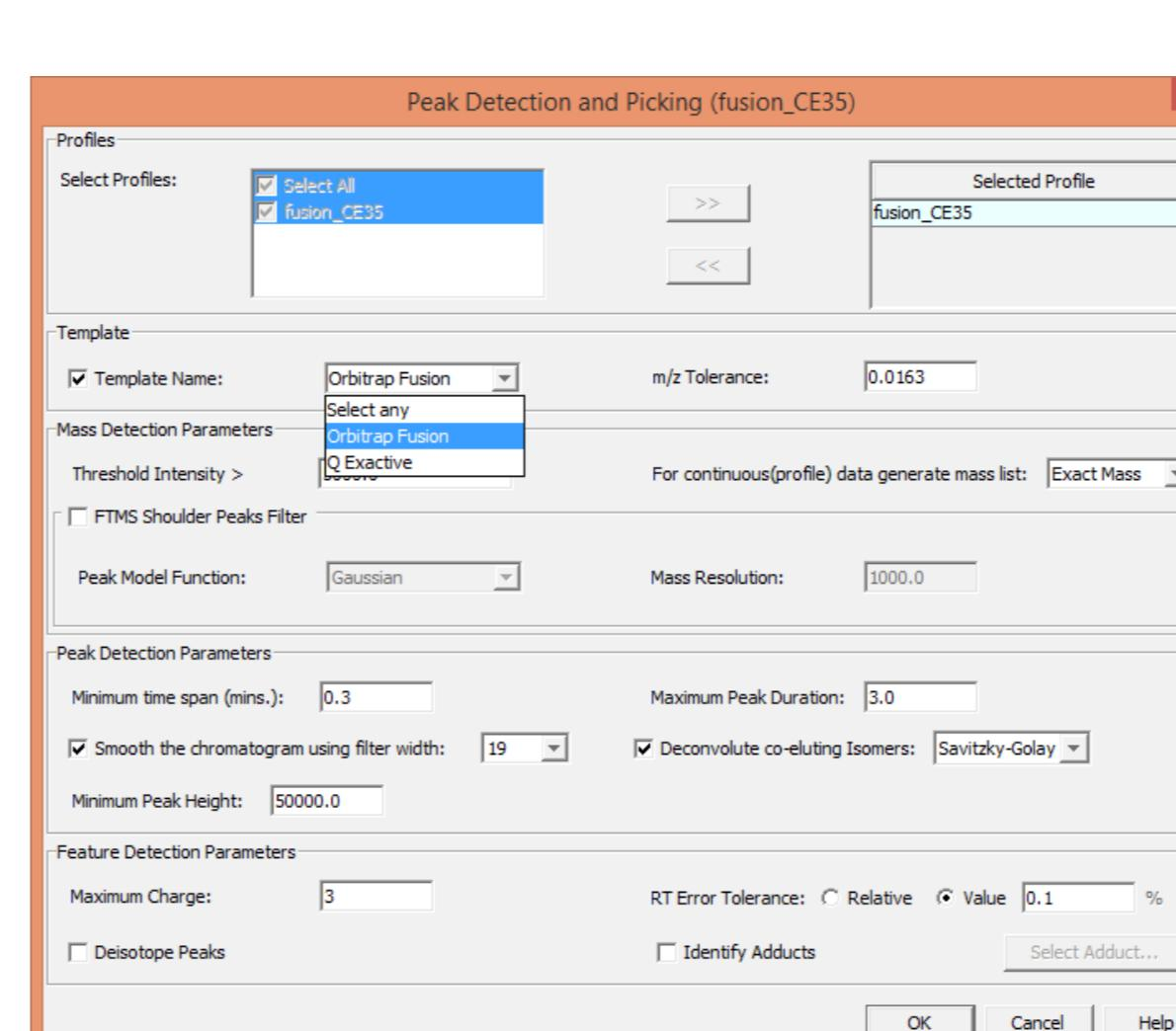
Figure 5: Shows a typical graphical user interface of SimGlycan software facilitating selection of peak detection and picking templates based on instruments.
